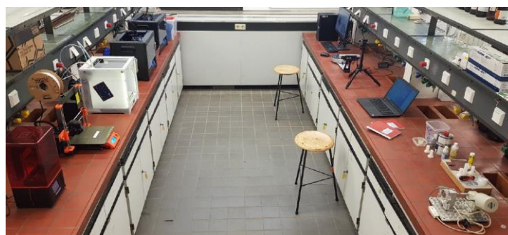
Figure 2. A two-bench 3D-lab for teaching and applications: DLP-printer, open FDM and three closed FDM printer, 3D scanner with camera and flow-reactors as printed from these printers (from left to right).
