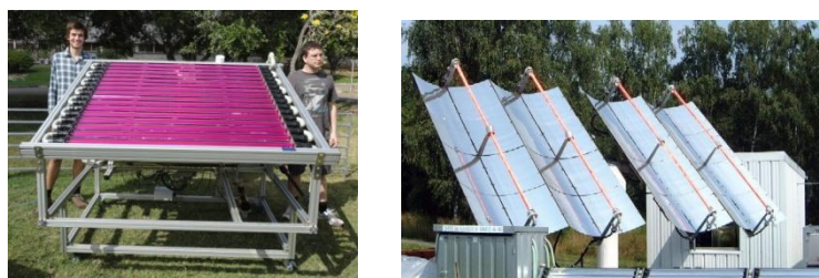
Figure 3. Solar CPC reactor at JCU (Australia) and PROPHIS plant at DLR (Germany).
