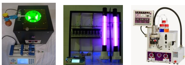
Figure 4. Continuous-flow photoreactors and Vapourtec's UV-150 module.
