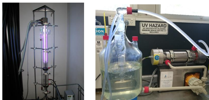
Figure 2. Vertical falling-film (University of Cologne, Germany) and horizontal loop reactor (JCU, Australia).
