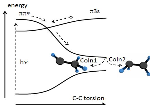
**Figure 1.** Sketch of the dynamics of ethylene upon excitation to its lowest lying  $\pi\pi^*$ -state.
